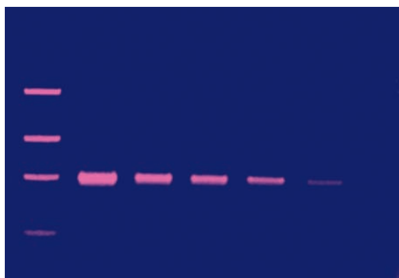
Figure 5.1 DNA gel electrophoresis. (a) Scheme of the method: This is a horizontal gel made of agarose (a substance derived from seaweed, and the main component of agar). The agarose melts at high temperature, then gels as it cools. A “comb” is inserted into the molten agarose; after the gel cools, the comb is removed, leaving slots, or wells (orange). The DNA is then placed in the wells, and an electric current is run through the gel. Because the DNA is an acid, it is negatively charged at neutral pH and electrophoreses, or migrates, toward the positive pole, or anode. (b) A photograph of a gel after electrophoresis showing the DNA fragments as bright bands. DNA binds to a dye that fluoresces orange under ultraviolet light, but the bands appear pink in this photograph.
